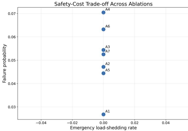
Fig. 12. Safety-cost trade-off across ablations: failure probability versus emergency-shedding rate. The complete method (A7) attains low failure probability without resorting to costly shedding.
