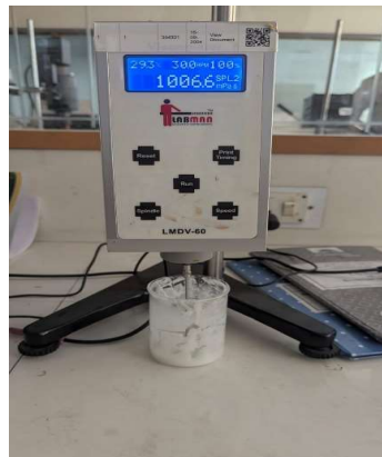
Figure 5.5:- Determination of Viscosity of formulation batch F1 and F3
