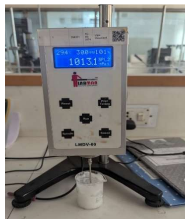
Figure 5.5:- Determination of Viscosity of formulation batch F1 and F3
