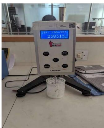
Figure 5.5:- Determination of Viscosity of formulation batch F1 and F3
