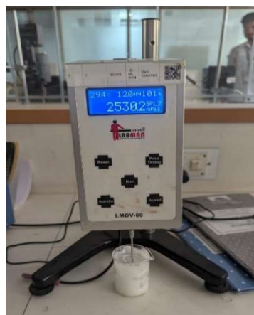
Figure 5.5:- Determination of Viscosity of formulation batch F1 and F3
