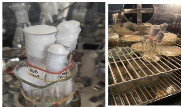
Figure 2. Cotton-plugged nutrient broth tubes during the alternating incubation cycle: (left) secured upright on the orbital shaker during the daytime agitation phase; (right) transferred to the static incubator (37 °C) overnight. Visible turbidity at the tube base reflects progressive bacterial growth.
