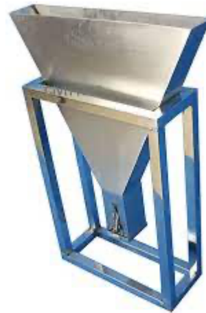
Fig 3. V-funnel test equipment (Rectangular section Equipment)
