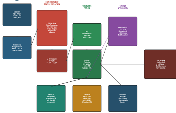
Figure 1. DINOv2-KMeans Architecture: PathMNIST patches processed through DINOv2-Base feature extraction, L2 normalisation, PCA compression (768-D \rightarrow 128-D), multi-criterion K optimisation ( K=2-10 ), and K-Means clustering ( K=5 optimal). UMAP, evaluation, and representative patch modules complete the pipeline.
